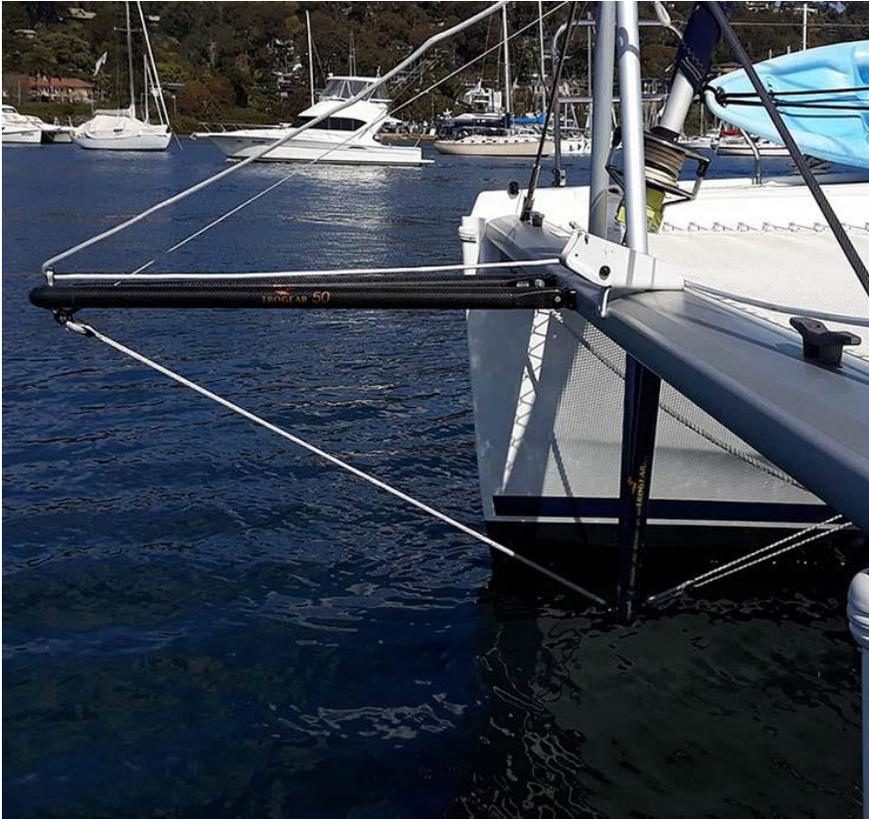
You can also install using a second, shorter sprit as a dolphin striker. With this set up, you do not need whiskers. The benefit of this system is to avoid any conflict with whiskers when deploying an anchor. Additionally the bobstay in this solution works better due to a better pulling angle and less flexing compared to bridle/whiskers.
